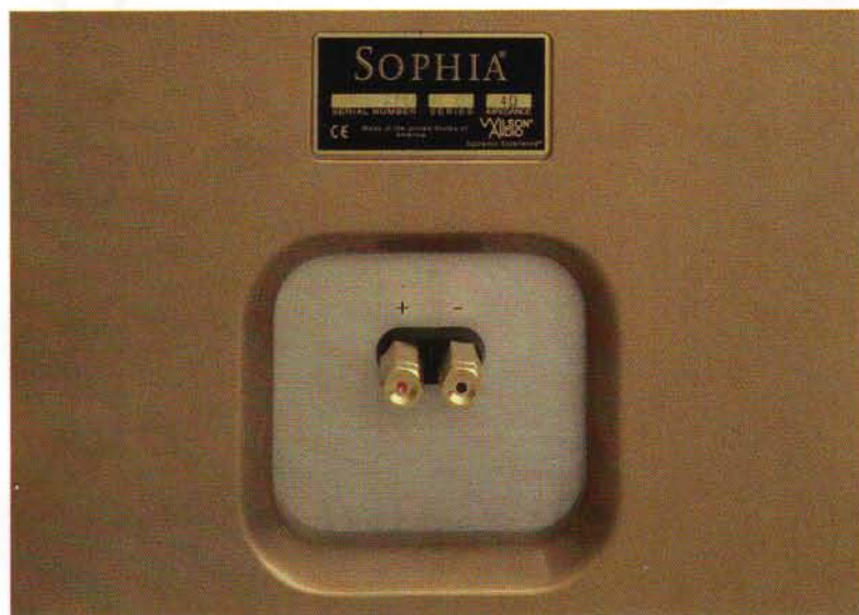
ABOVE: No bi-wiring here, just a stout pair of custom-made terminals, which can be tightened securely with a supplied hex tool. Badge clearly states 4ohm impedance!
